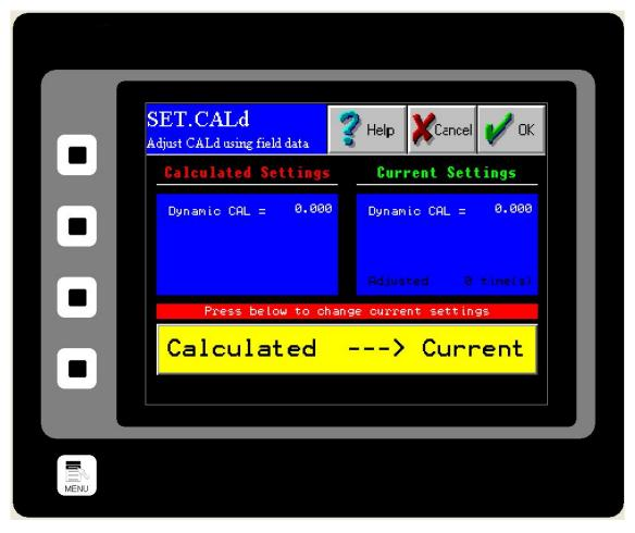
**Step 11:** To accept the new Dynamic Calibration press the YELLOW CACULATED to CURRENT Button and press the OK Button. A pop up screen will appear, asking if you are sure you would like to accept this value. Press YES.
