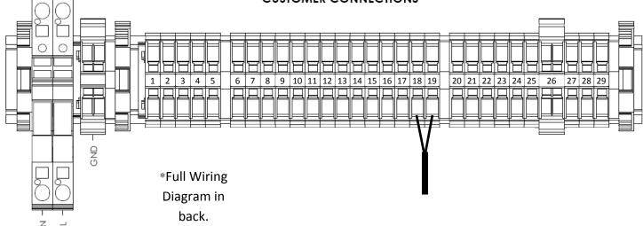
All Connections are made to the Bottom of the Terminal Blocks
