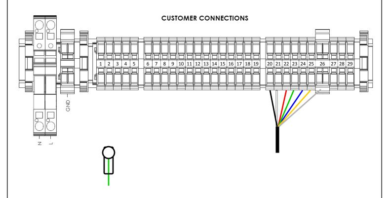
\*All Connections are made to the Bottom of the Terminal Blocks
