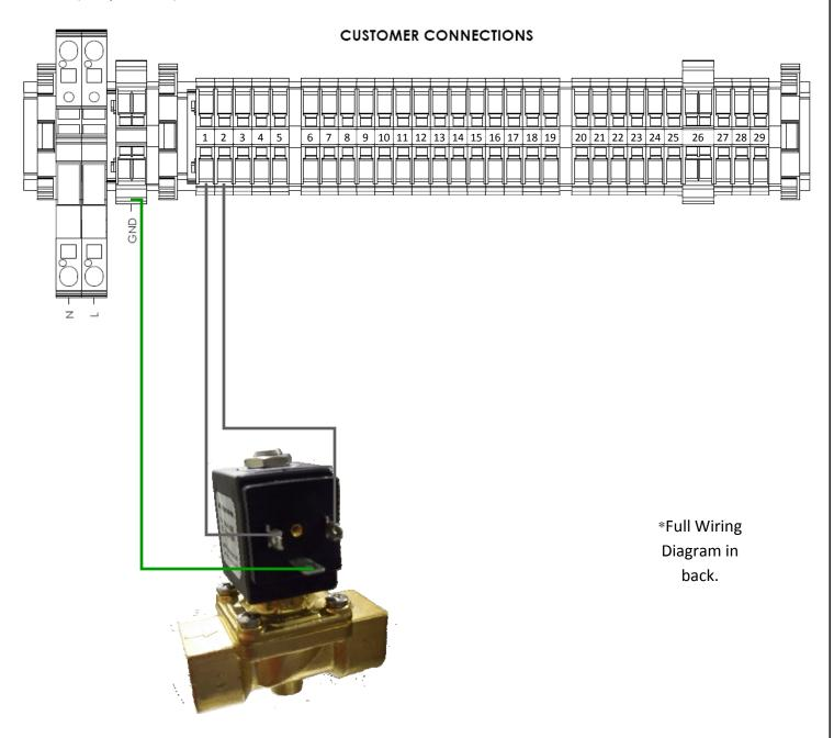
All Connections are made to the Bottom of the Terminal Blocks
