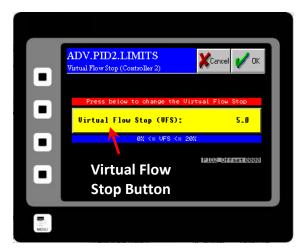
Virtual Flow Stop™ is typically set by increasing the Manual Valve until flow just begins to trickle from the valve and then, set the Virtual Flow Stop™ to 2/3 of that value. This value is, of course, dependant on the particle size and characteristics of your product.
