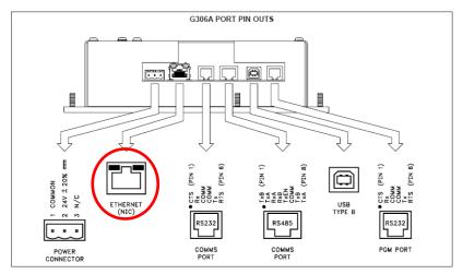
Step 2: You must first Manually Configure the IP Address for your Digital Electronics. In order to accomplish this, you must first access the COM.IP page by pressing the COM Button on your TOP Menu and then, pressing the IP CONFIG Button. You should now see this screen (right).
