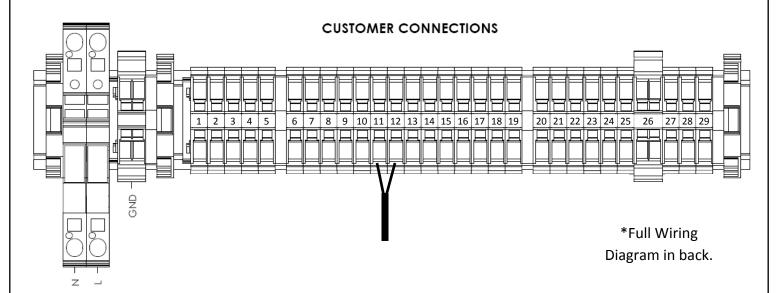
\*All Connections are made to the Bottom of the Terminal Blocks
