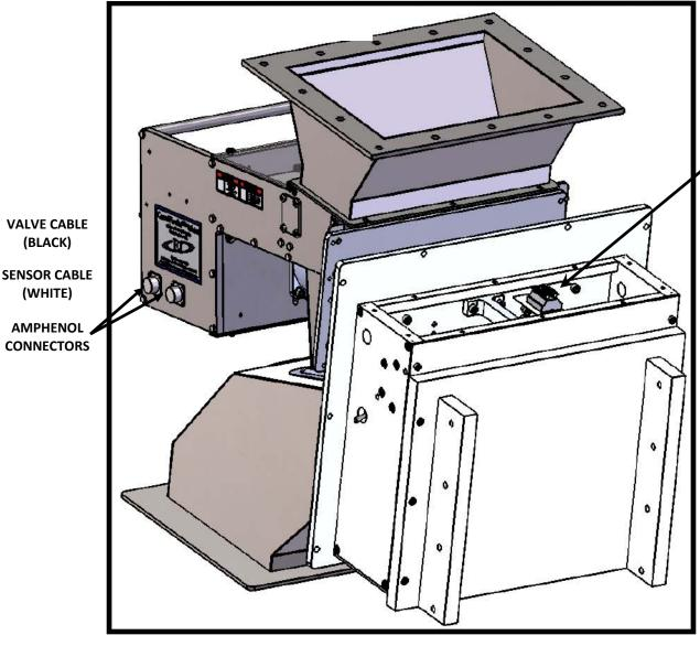
Please be sure to ground the Wago Connector for the Transducer. To do so, run your ground wire, along with the Transducer Cable, through the Customer Provided Conduit and Connect to both the Meter and The Digital Electronics as shown. The Ground Wire should attach to both the Ground Screw on the Wago Connector Mount (Above) as well as to the Ground Lug within your Digital Electronics (Right).
