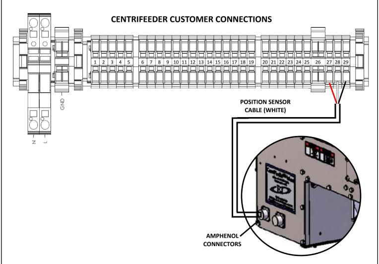
\*All Connections are made to the Bottom of the Terminal Blocks
