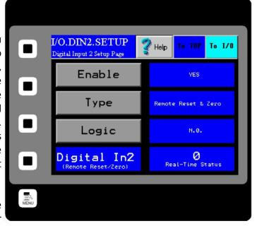
The logic of the Remote Reset Capability can also be manipulated. If the LOGIC Button is pressed, a dialog box will prompt you to chose from two options, "NC" or "NO". The options are described below.
