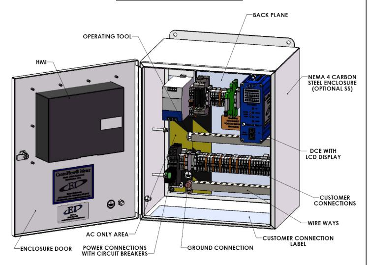
The Digital Electronics Enclosure contains the HMI, the Digital CentriFlow® Electronics (DCE), Power Supply, Alarm Relay, Power Connections with Knife Disconnects, and the Customer Connections.
