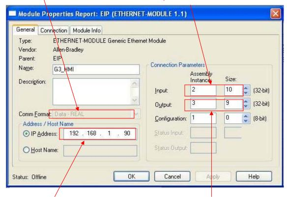
The IP Address is the address of the HMI. This must be the same as the address set in the HMI.
