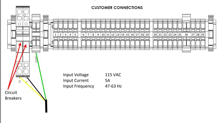
\*All Connections are made to the Bottom of the Terminal Blocks
