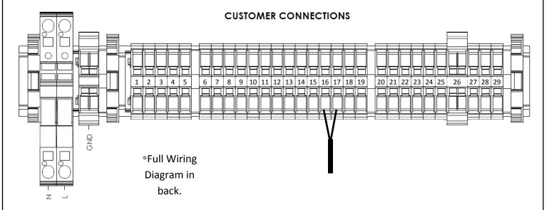
All Connections are made to the Bottom of the Terminal Blocks
