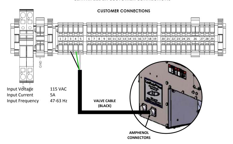
\*All Connections are made to the Bottom of the Terminal Blocks
